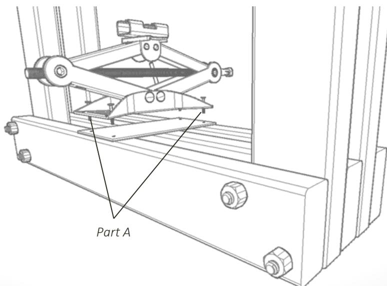
**Step 3:** Use 2x PART H for a stand. The two sheets of plywood should be cut to 560mm length and 360mm height. You will need to drill about 6 holes in each and attach them using PART A. (see 1d)
