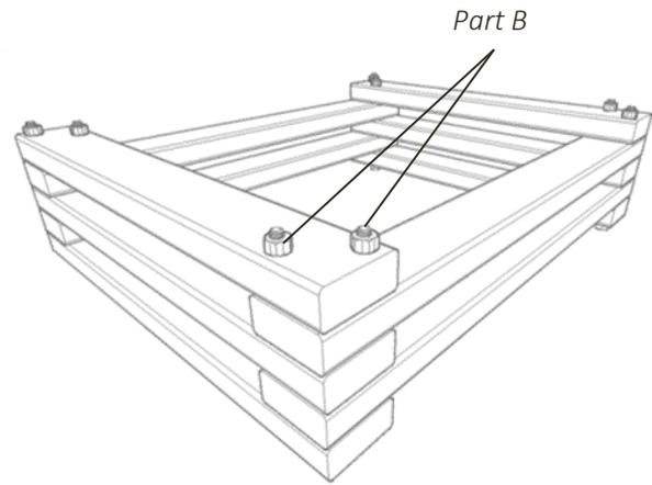
**Step 2:** At this point you can fit your car jack (PART K) to the frame. If the base of your jack is not the right size to fit the frame, you will need to attach the jack to a steel plate (PART I) prior to fixing it to the frame. Drill holes into the base of the car jack for the screws (PART A).
