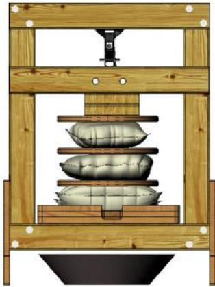
*The car jack is slowly turned creating downwards pressure and squeezing juice out of the pulp filled muslin pouches.*
