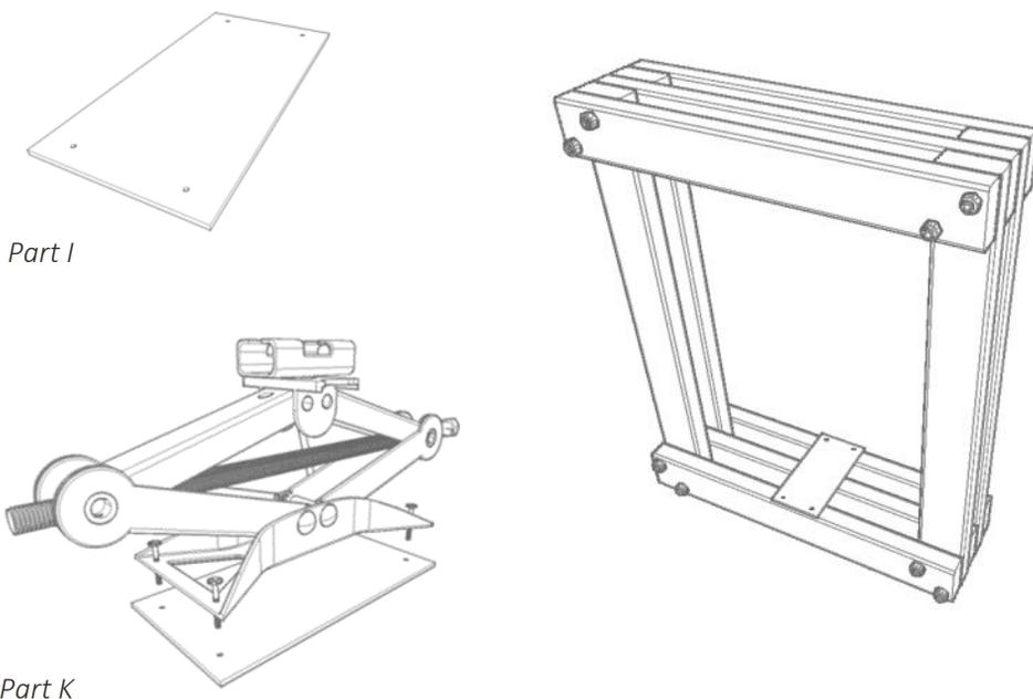
Attach the car jack to the frame of the cider press using screws as shown below;
