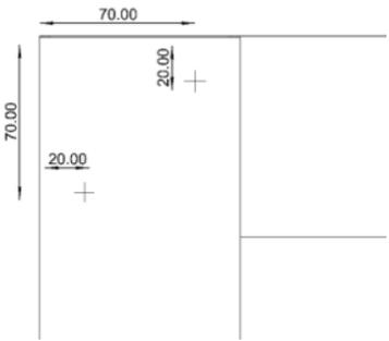
Mark two holes at either end of each plank at the points shown above.
